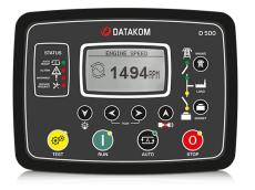
Main Status and instrumentation display Alarm LED's Close generator button Status LED's Operation selecting buttons
